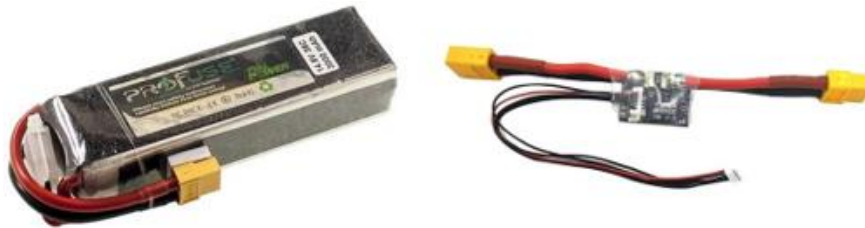
Figure 9: LiPo battery and power distribution module
